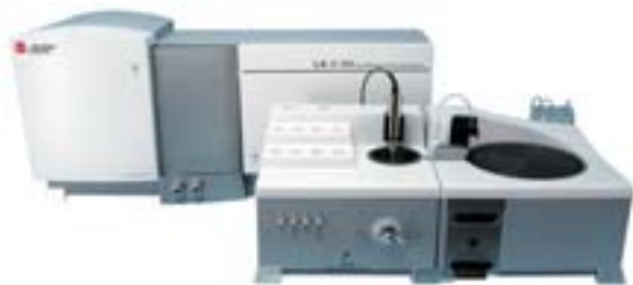
Figure 1. Beckman Coulter LS 13 320 Particle Size Analyzer with the Aqueous Liquid Module (ALM) and the Auto Prep Station.
